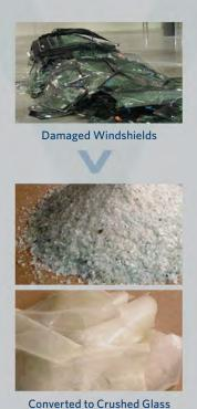
Converted to Crushed Glass Cullet and Recycled PVB Flakes
